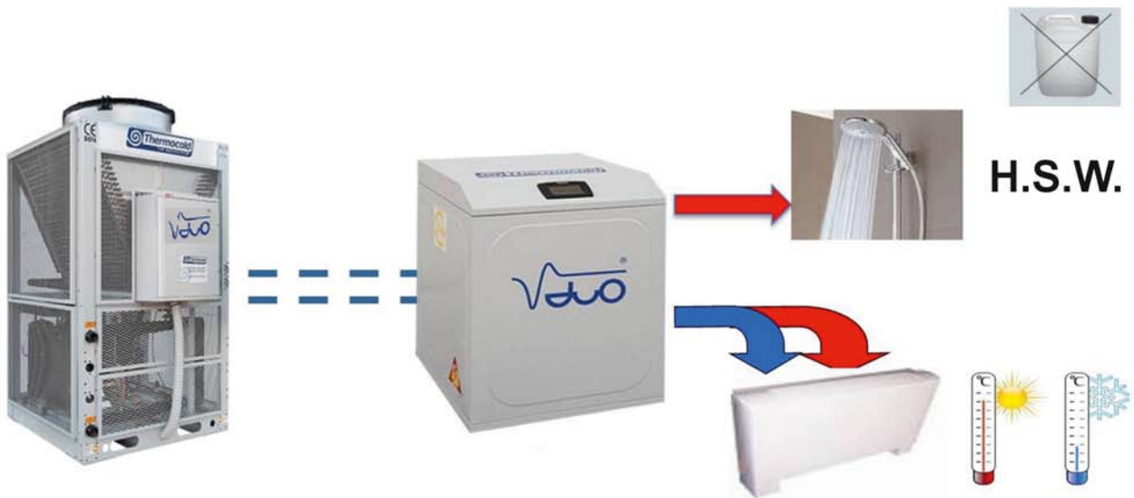
Figure 4. Split version of DUO® DUO® heat pump system.
